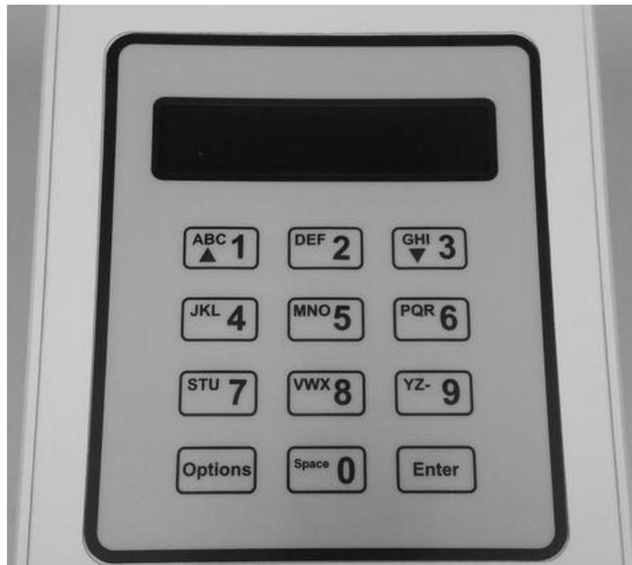
Figure 1-1 SAFE Sens IVM keypad and display
